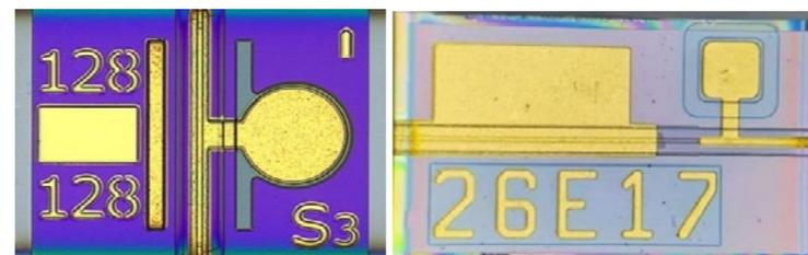
● 25Gb/sDFB 芯片 (250μm\*160μm)
