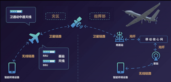
大型固定翼无人机应急通信系统架构图 The architecture diagram of China Mobile's UAV emergency communication system
